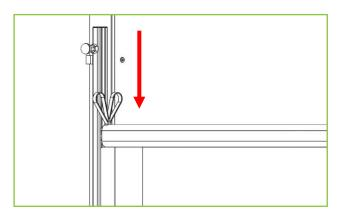
4. Make sure the siderail is fully down and top bar is below the top of the mattress at both ends. If SDR-0-FL4-000 is fitted, ensure the top bar is located properly by the bottom plunger. You may need to pull the plunger out, then push the siderail bar down and into the plunger.
