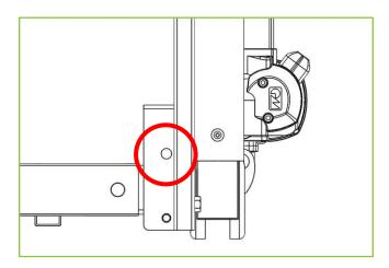
9. Fit the locking pin and R-clip. (50mm Long, supplied with the siderails).
