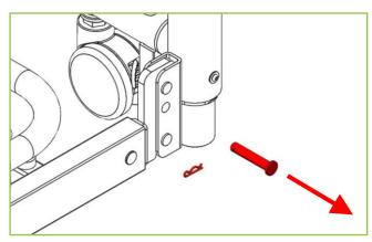
**Note** – This pin will not be needed to fit the siderails. Store safely for use should the siderails be removed.
