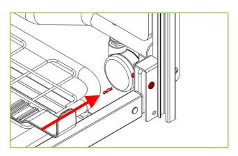
Fit the Bracket Fixing Screw (35mm long) using a 5mm Allen key.
