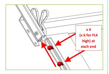
**Note** – Siderail SDR-0-FL4-000 and SDR-H-FL4-000 has an additional locking plunger at the base of the support. Pull this plunger out in order to move the bars up the sliding track.
