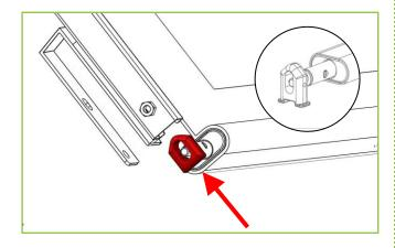
22. Fit the Bottom Bar Fixing Screw (25mm long) using a 5mm Allen key.
