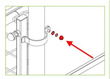
13. This bracket is now in place. Repeat the above process to fit a siderail bracket to the right-hand side of the bed at the head end.
