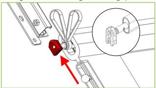
20. **Important!** Ensure **ALL** the plastic guides are fitted into the sliding track. (4 Plastic guides each end of siderail fabric – 6 each end for FL4 high)
