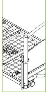
**Note** – If bumpers are fitted, the bracket cannot be slid down the tubular bed support. Locate the base of the bracket on the mattress platform, then position the curved part of the bracket against the headboard.
