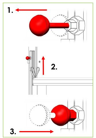
3. Ensure the siderail is properly raised and latched by pushing down gently.
