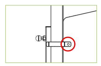
12. Fit the upper footboard fixing bolt and nut as indicated below using a 4mm Allen key and 10mm spanner. If Bumper Set BMHNE-0-FL4-000 is fitted, ensure that no material is pinched in the bracket.
