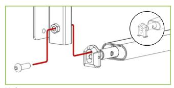
**Note** – once the bottom bar fixing screw has been fitted, make sure the bottom bar cannot move up or down.
