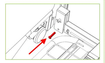
11. Align the hole of the curved part of the bracket with the hole in the footboard.
