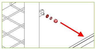
5. Remove the mattress platform locking pin and R-clip.
