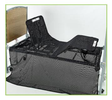
5) Take the long flap of material from the side of the safety sleeve and take it under the bed frame, zip it onto the short flap of material ensuring that any cables are enclosed by the safety sleeve. Leave the head and foot ends unzipped; they will be zipped later in the fitting sequence.
