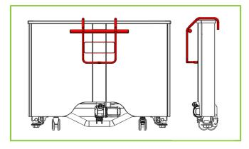
4. Use the pump hanging brackets to fit the pump:
