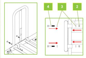
6. Cap the head of the bolt with the bolt cap.
