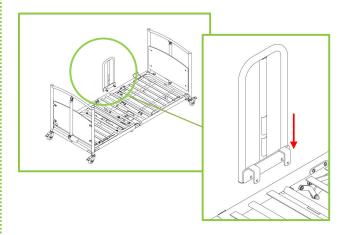
Clamp the CommunityBed Bed Lever to the frame of the Community Bed with the bolts, washers and nuts. Tighten the nuts and bolts with the 13mm spanner.
