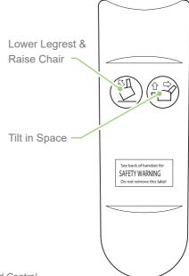
Figure 22 - Two Button Hand Control
