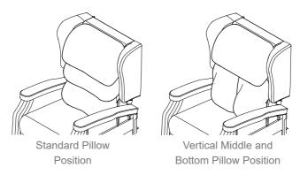
Figure 11 - Fitting / Adjusting Backrest Pillows
