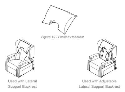
Figure 20 - Profiled Headrest Examples
